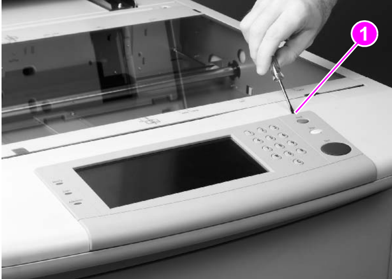
Figure 62. Control panel (1 of 3)
